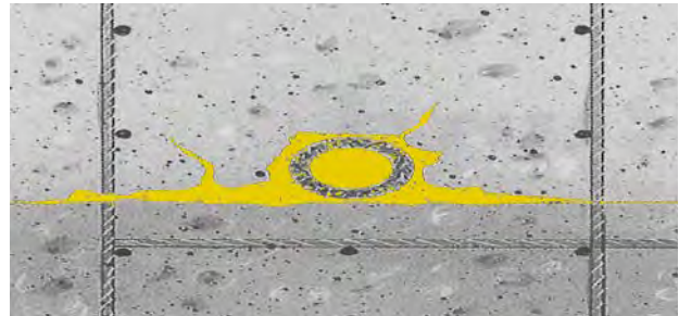
Leakage sealing by injection
